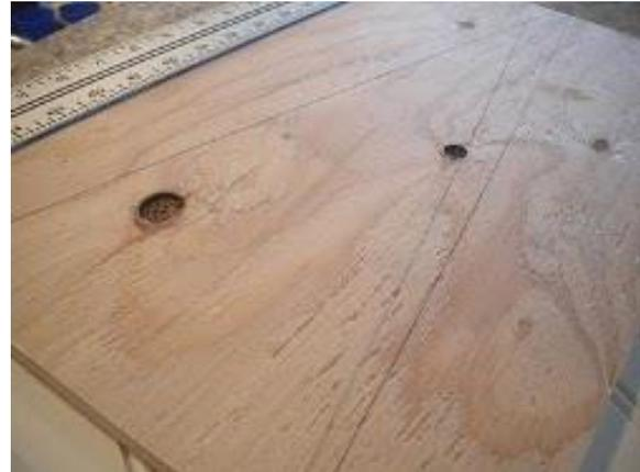
2.) Cut your triangle piece out with a Bandsaw, Jigsaw or Circular saw.
